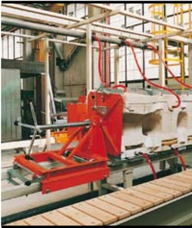
In this system, too, traditional battery casting simplifies every processing phase. This system enables to simultaneously produce bowls and bidets in up to 80 moulds. The mould carriages slide on 2 benches and final extraction is carried out mechanically. Thanks to an LCD and PLC, the production cycle variables can be viewed and controlled.
