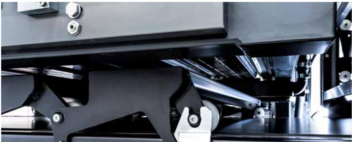
Automated ink reservoirs also allow collection of spitting and purge cycle residues, thus avoiding any staining of the belt and the consequent dispersion of inks into the environment. An independent dual cleaning system with extraction bar aids cleanliness of the active module during routine operation.
