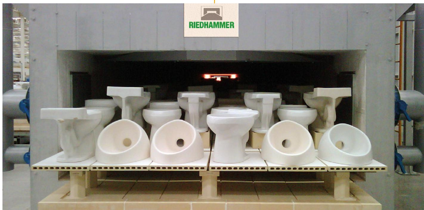
al production requirements. One interesting approach to flexible production involves designing **continuous kilns capable of operating using only part of their installed capacity.**
