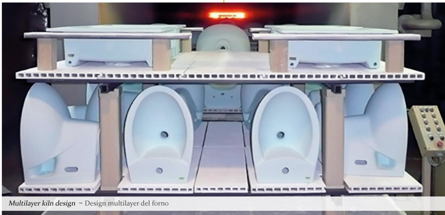
Multilayer kiln design ~ Design multilayer del forno
