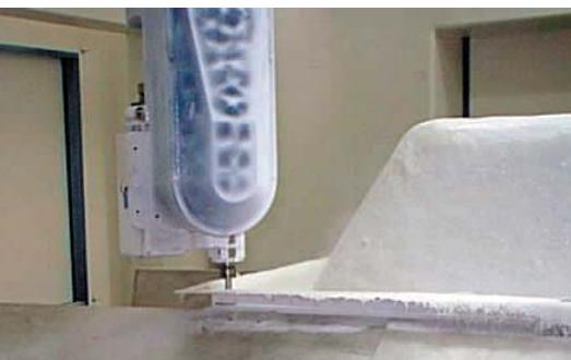
Placed just after the dryer and introduced in a properly sound-proofed booth, this machine allows the bathtubs cutting and drimming directly on the plant of the fiberglass spraying. The different models of bathtubs and shower trays are suitably positioned by a centering device while a portal unit complete with a cutting tool provides for the edges cutting. Drilling of the "overflow" is carried out by a tool change.
